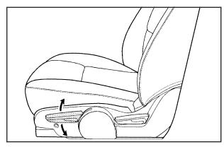
If your vehicle has a manual driver seat height adjuster, it is located on the outboard side of the seat near the front of the seat cushion. To raise the seat, move the lever upward repeatedly until the seat is at the desired height. To lower the seat, move the lever downward repeatedly until the seat is at the desired height.
